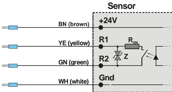
For signalling, a semiconductor relay is used whose galvanically decoupled switching output has a maximum permanent switching power of 300 mW (at an  $R_{on}$  of typically 20 to 25  $\Omega$  max.). The switching current should be at most 100 mA, the peak value of the switching voltage (AC or DC) must not exceed 30 V, since otherwise the bidirectional protecting diode (Z) between the load circuit terminals will break down and can be thermally destroyed (see connecting diagram).
